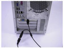
For TVs with Composite video inputs, attach the included S-Video to Composite converter adapter to the female 4-pin S-Video connector.
