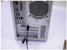
For TVs with S-Video inputs, connect one end of a standard S-Video cable into the TV and the other end into the female 4-pin S-Video connector.
