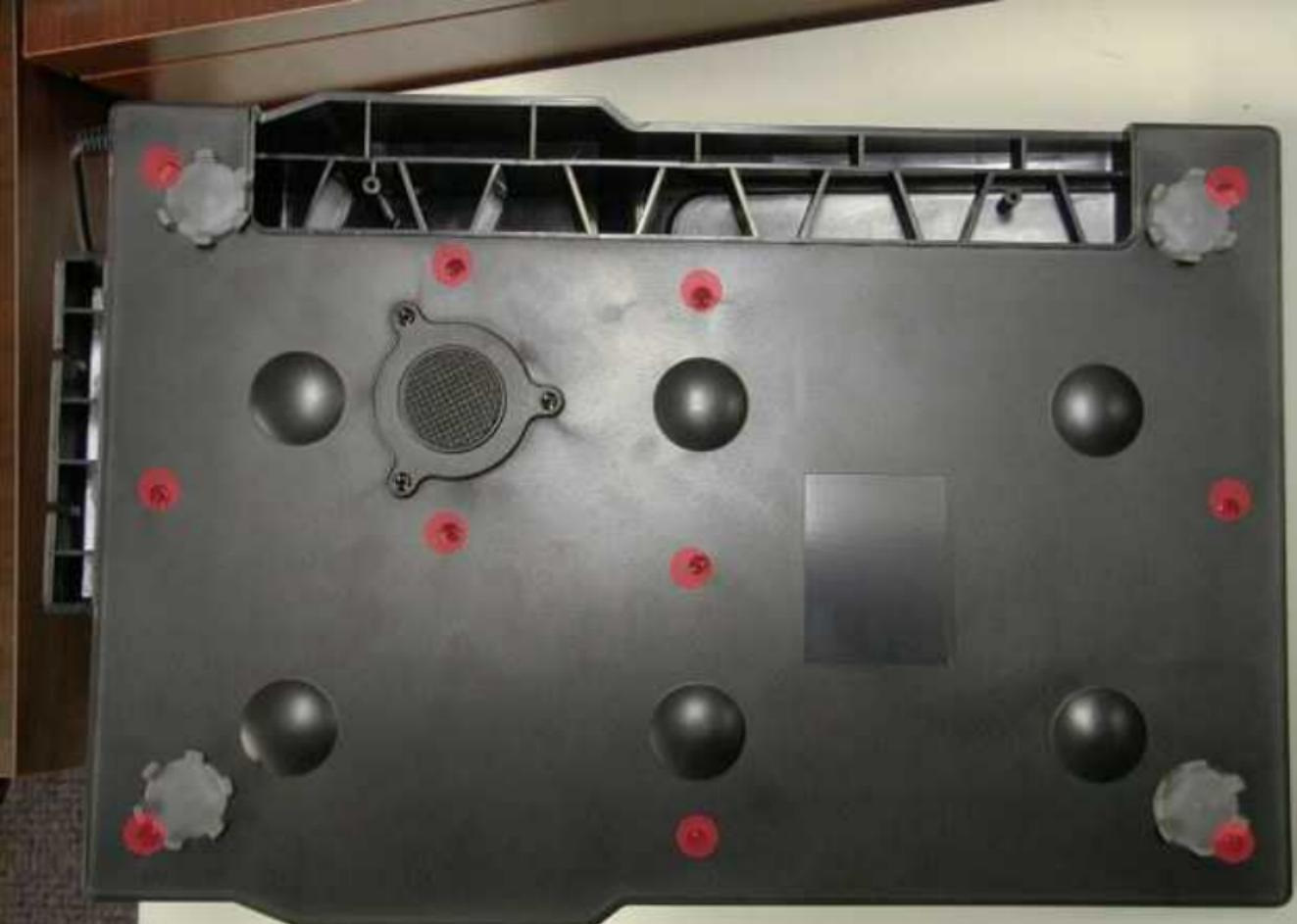
**Step 1 - Remove the 11 screws from the base.**
