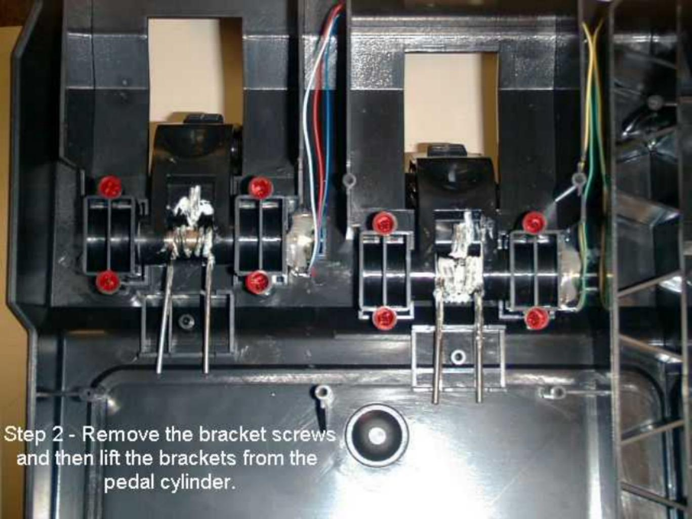
Step 2 - Remove the bracket screws
