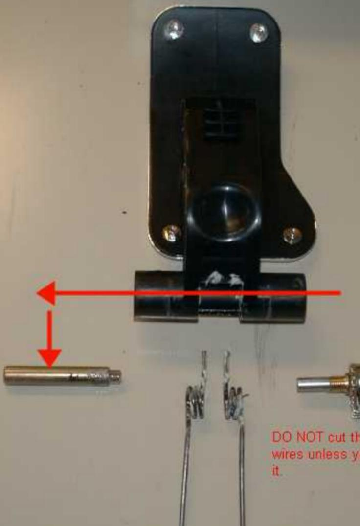
DO NOT cut the potentiometer wires unless you are replacing it.
